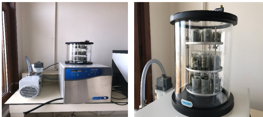
Figure 2: Images related to the drying of Stevia plant samples using a lyophilizer
