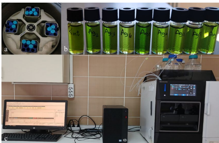
Figure 5. Following extraction for HPLC analysis, centrifugation of the samples (a), transfer into vials (b) and HPLC measurement/analysis (c)
