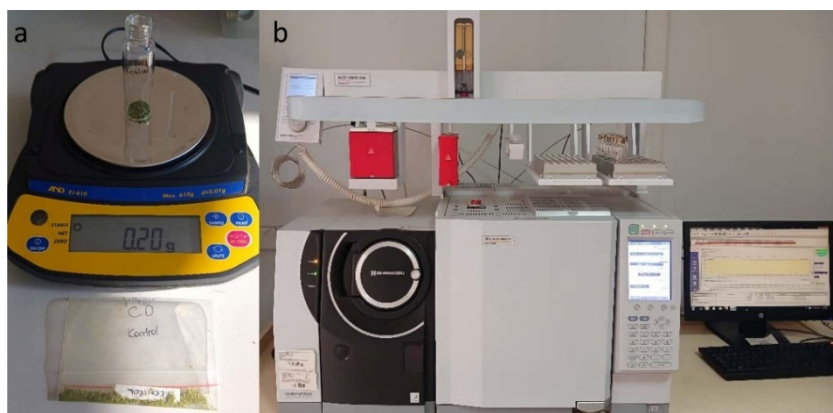
Figure 4. Preparation of samples for GC–MS analysis (a) and GC–MS measurement/analysis (b)
